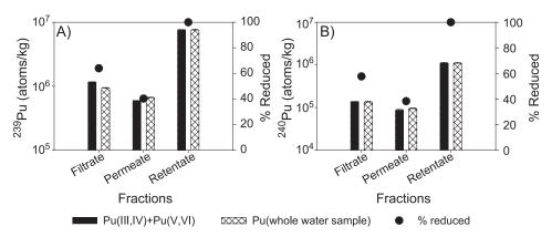
Fig. 4. Comparison of the sum of redox subfractions [Pu(III/IV)+Pu(V/VI)] and the independently measured Pu in whole water samples. Also shown is the percentage of reduced Pu(III/IV) in the filtrate sample fraction from well K-27.
