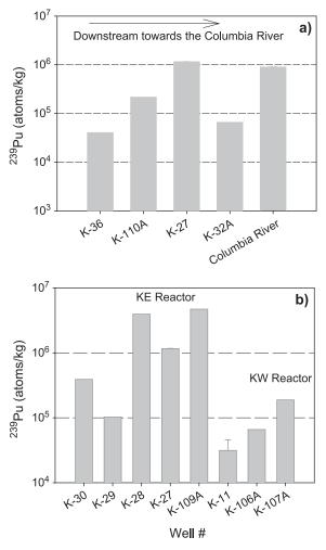
Fig. 3. <sup>239</sup>Pu concentrations in 100K-Area wells of the Hanford Site. Data include both collections in 1997 and 1999. (a) Transect following the groundwater flow towards the Columbia River. (b) Transect across the reactors.
